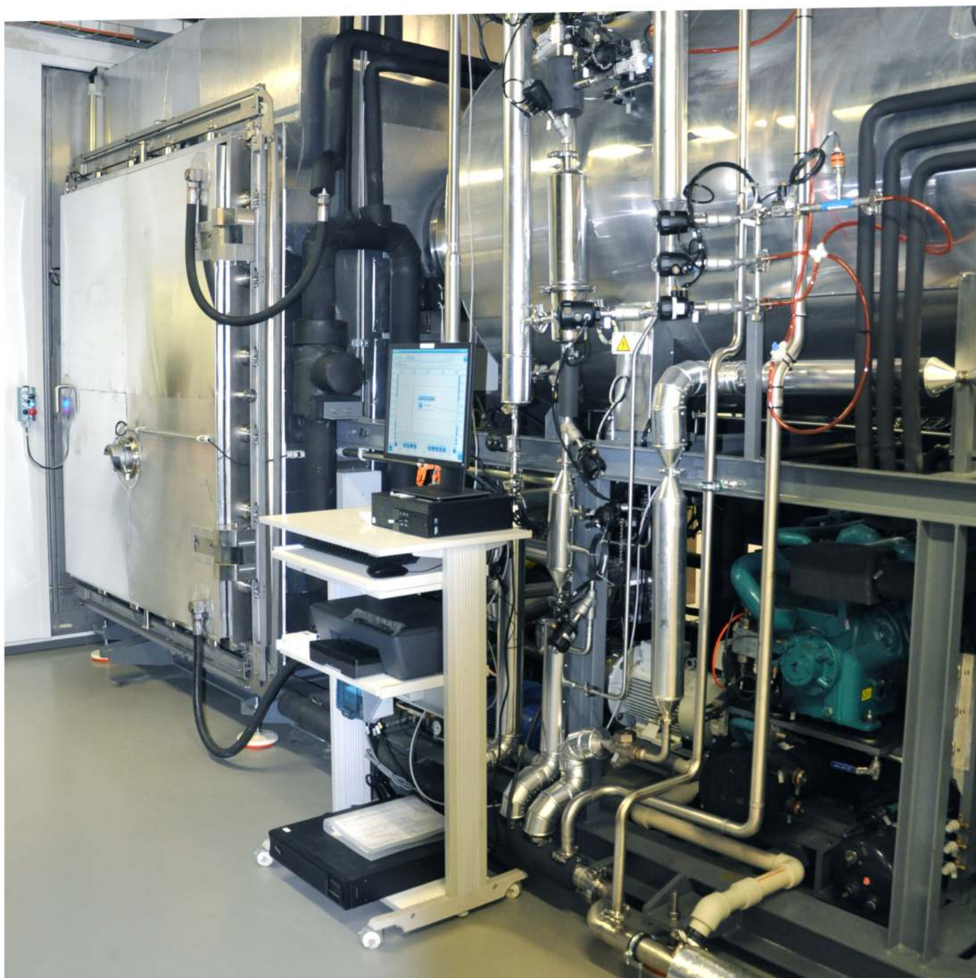
The modern lyophilisation device LYOMEGA 200 will amaze with its capacity of 110,000 pieces of phials with a volume of 3 ml and automation of the lyophilisation process, including the automatic system of setting up phials
