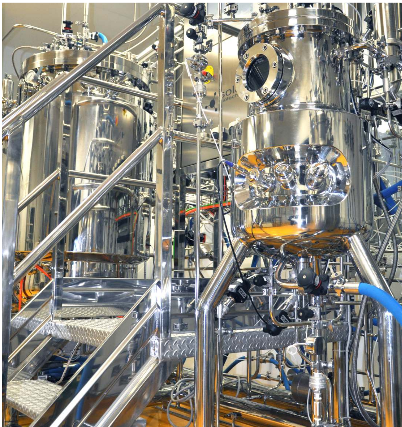
The SOLARIS SBI400 Bioreactor secures an efficient viral antigen cultivation process. The bioreactor has a working volume of 300 litres and produces a maximum of 600 litres of antigen containing glycoprotein (after inactivation) of 40-80 IU / ml per month
